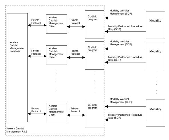
Figure 2. Xcelera Cathlab Management 1.2 in a DICOM network
